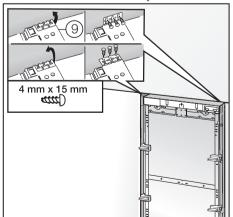
■ Pull out the lugs for the side fixing plates ⑨.
